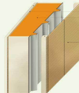
石灰抹墙 15mm lime plastering 15mm
